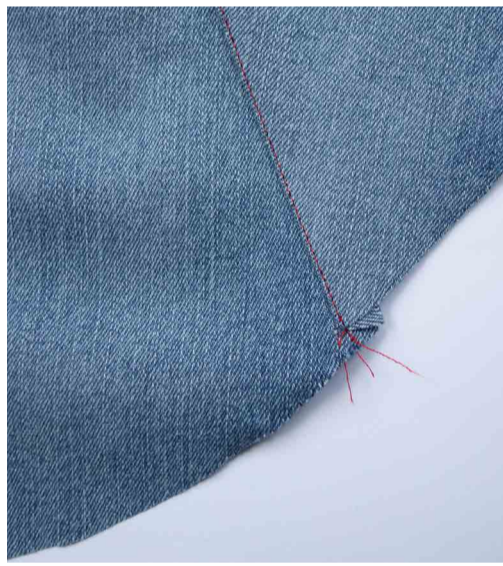
8. Sew the two pieces together along the bottom edge (Seamallowance 1 cm).
