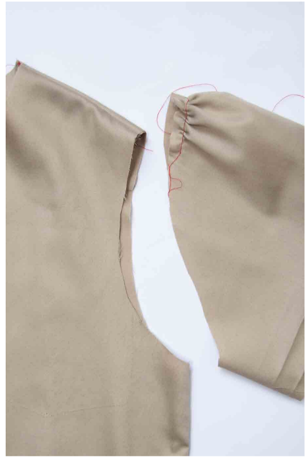
8. Lay the sleeve and the body so that the notch at the armhole and the sleeve align.
