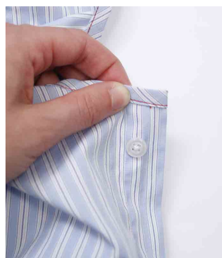
6. Similar to the bias tape on the other side of the collar, pin the tape to the inside of the garment.
