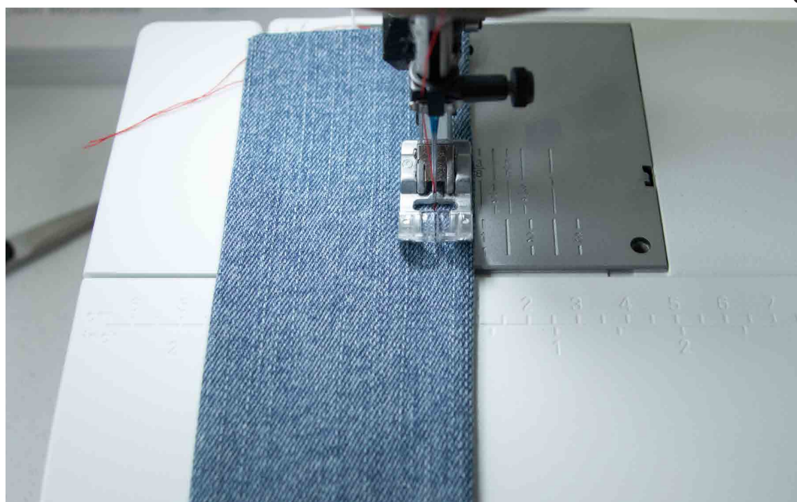
16. To make the straps stay in shape, you can topstitch the straps by sewing around the edge.
