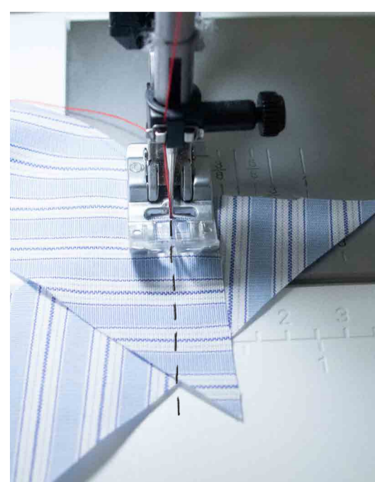
4. Sew the pieces together. Sew together about 3 - 4 stripes to have enough material for the collar.
