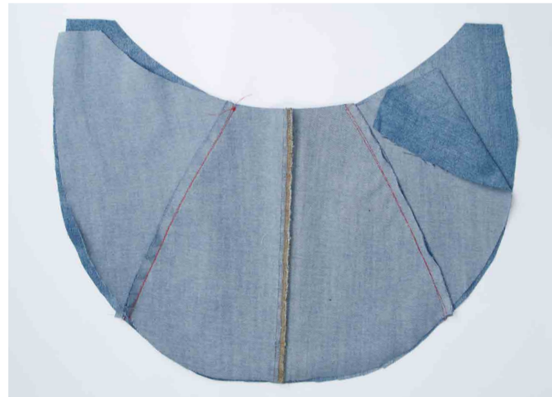
9. Lay the two sides of the body on top each other so that the right sides are facing each other, sew the two pieces together along the bottom edge (Seamallowance 1cm).
