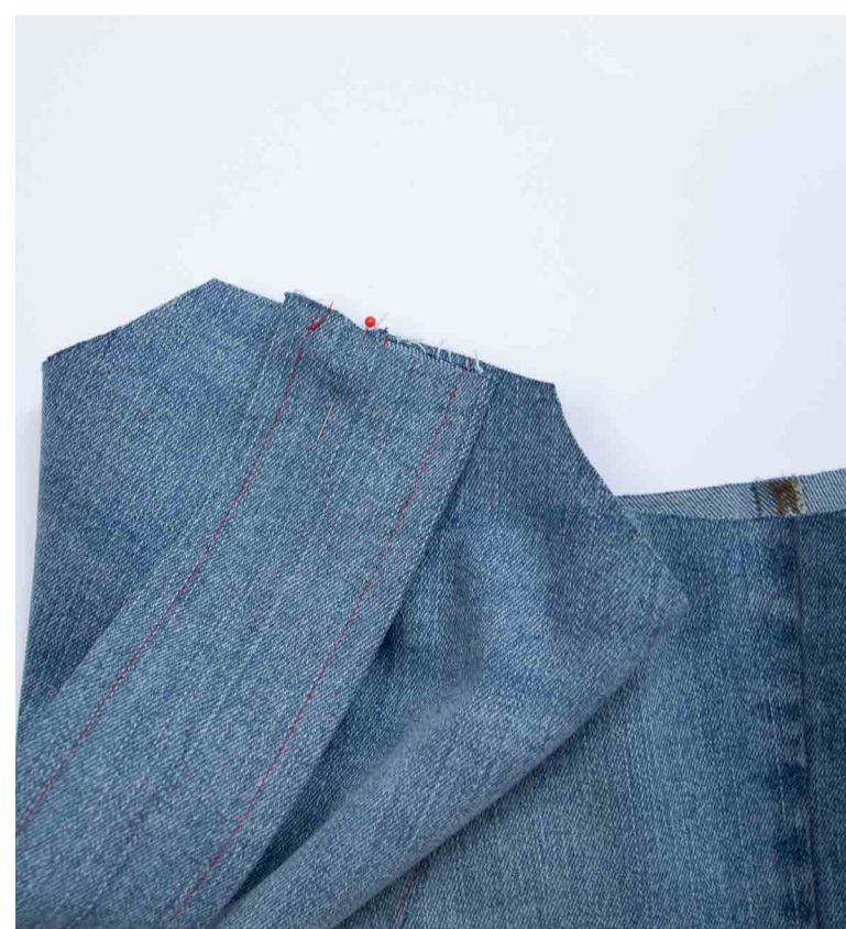
20. You can attach it with a pin before sewing.
