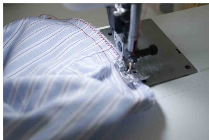
9. Cut away any seamallowance that might be more than 1cm. Then, with the zig zag stitch of you sewing machine finish the edge of the seamallowance.
